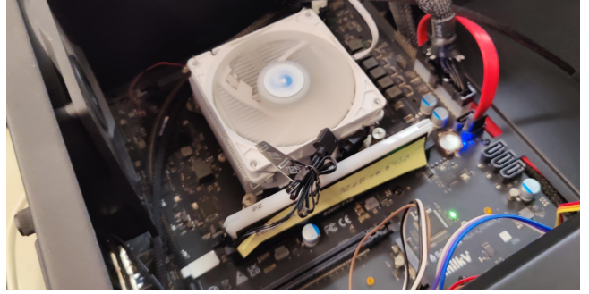
Figure 2: Experimental setup showing off-the-shelf Milk-V Pioneer motherboard, including Sophon SG2042 RISC-V CPU (top, under fan) and single DDR4 DIMM (bottom) with unlocked SPD.
